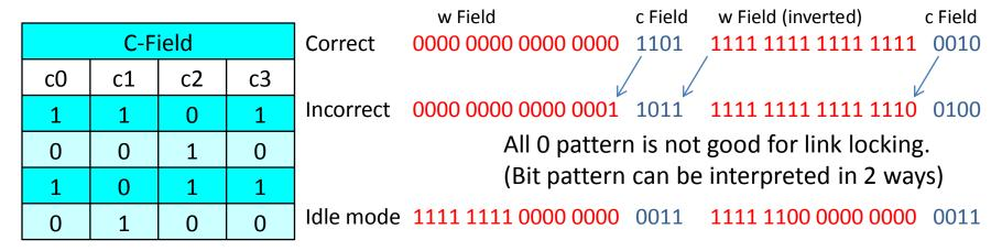
Synchronization process in sending idle words solves the problem, and the procedure has been implemented in ATLAS DAQ framework.
