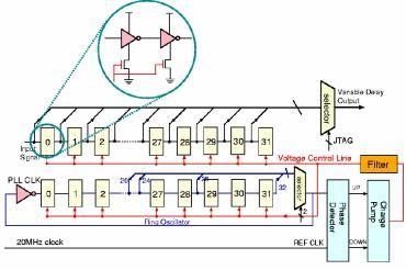
32 step variable precise delay with PLL circuit (1Step=25ns/28)
