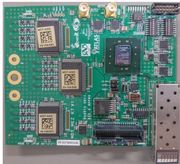
Trigger processor board
