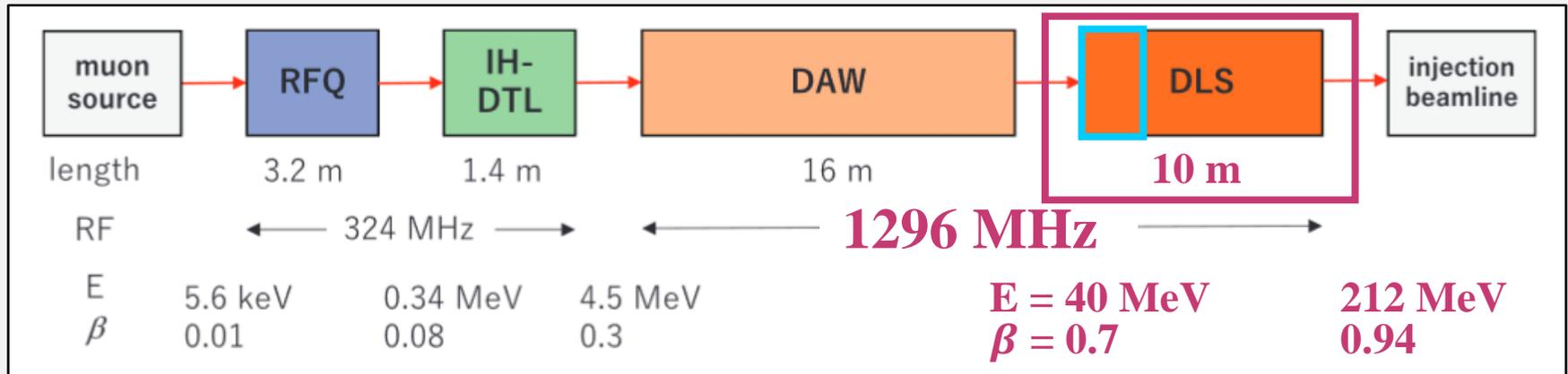
Schematic configuration of the muon LINAC [4].
