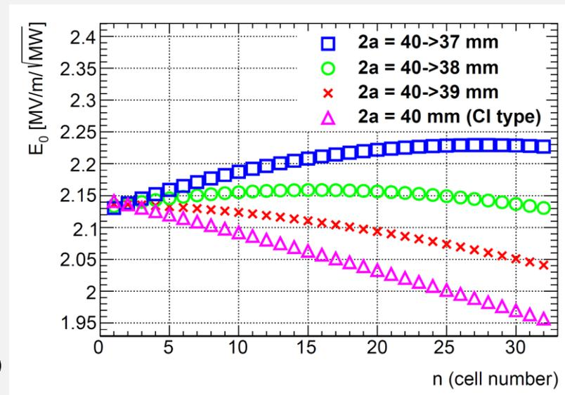
**The structure with  $2a_{\text{last}} = 38$  mm (green) has the most uniform gradient.**
