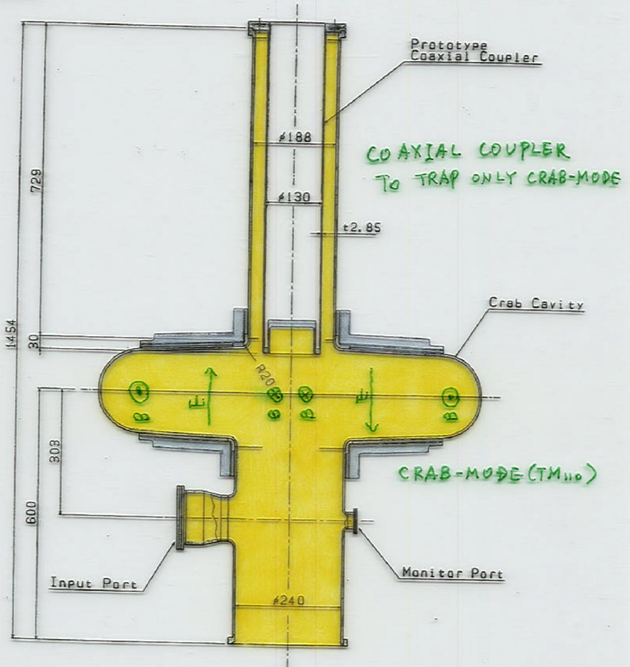
Cross section of the Crab Cavity with the Prototype Coaxial Coupler
