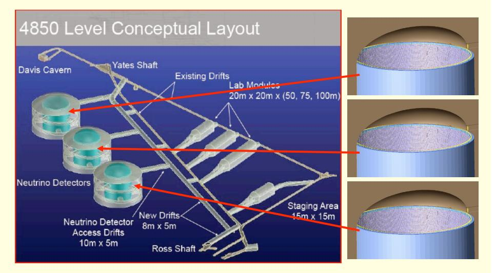
25% PMT coverage  $\rightarrow$  60,000 10 inch PMT's per module
